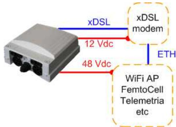
The RPW (power card of DataPowerBoost) can connect a modem and a data collector/distributor device. These units can be housed in the same box or can be installed in close boxes like DPs or cabinets.
